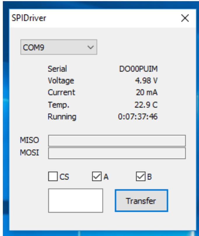
If there is only one serial device, the SPIDriver device should be automatically selected. If there is more than one device, select its COM port from the pull-down menu at the top. Once connected, you can control the signal lines and transmit hex values.
