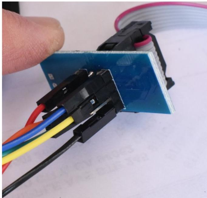
and connect the clip cable pins to the SPIDriver like this:
