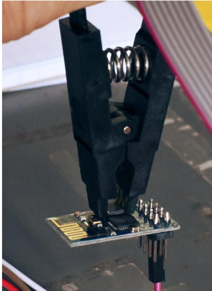
For the ESP8266, the CPU needs to be kept in reset so there is no contention while SPIDriver is driving to the flash. Connect SPIDriver's A signal (purple) to the ESP8266 reset:
